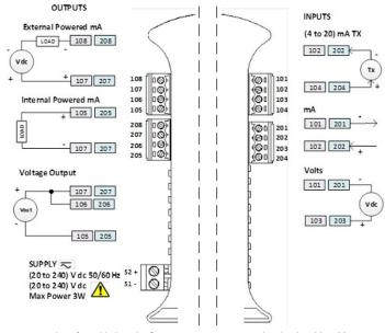
Input connections for cable length >3 metres: use screen or twisted pair cables. Max cable run 30 metres.
